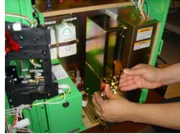
4. Lift up and release the cartridge. In some cases the bottom-most card will be stuck but proceed to lift up the cartridge. Afterwards, remove the jammed card.
