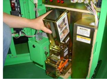
5. Reposition the cartridge. Align the cartridge with the  $\triangle$  symbol by pushing firmly from above. Then pull the cartridge forward with both hands as shown in the picture.
