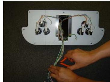
5. Unfasten the 4 carriage bolts and 4 flange nuts holding the card reader bracket in place and remove the card reader from the control panel.
